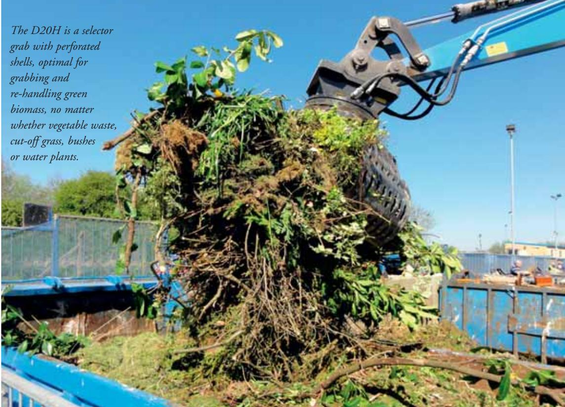
like water plants, the selector grabs of KINSHOFER's D-series are ideal. The shells are perforated to let water, dust and gravel through; for excavators with an operating weight from 1t to 80t.
