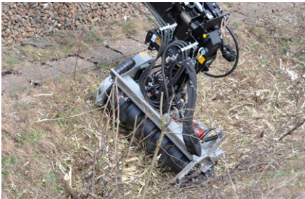
KM 931 mounted to a crane arm on a maintenance wagon (here with a mulcher)
