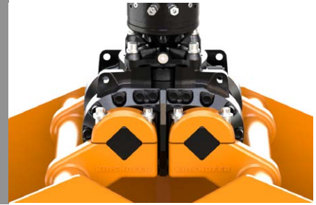
Loosen 4 bolts on each side
